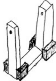
Step 6: Take out the base beams. Mark the center of the beams like this:
